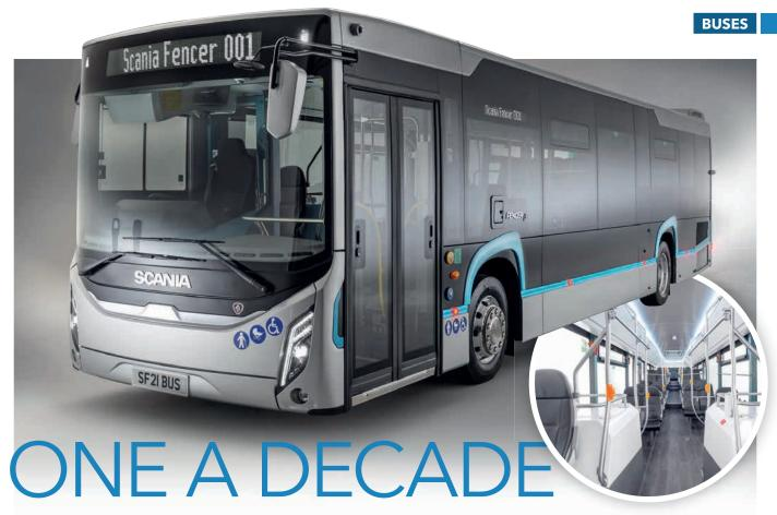
he line-up will encompass double-deckers and artics along with single-deckers, with the first battery-electric models scheduled to appear on this side of the Channel late in the first quarter of 2022, or early in the second quarter. They will be fitted with a 300kW electric motor driving through a two-speed gearbox and powered by either eight or ten lithium-ion batteries. The manufacturer was unable to give details of the range between recharges at the time of writing.
